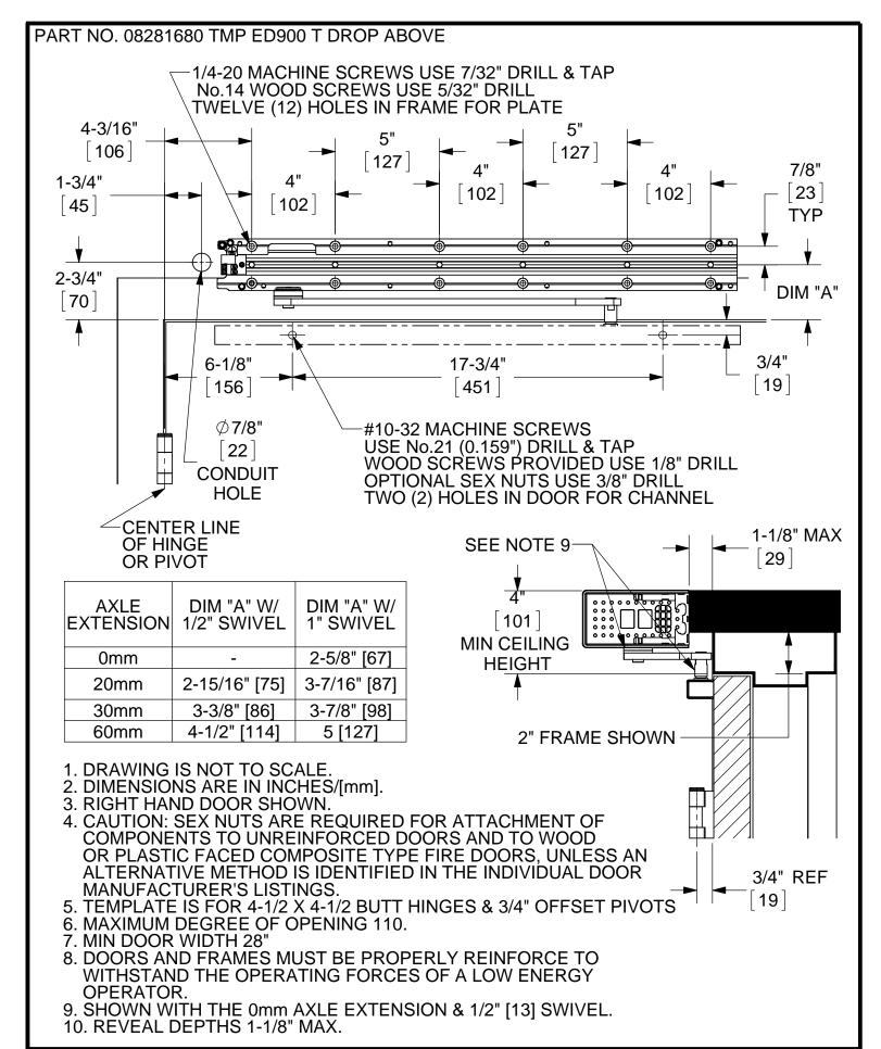
ED900 T TRACK INSTALLATION - PULL SIDE MOUNT DROP ABOVE 2" FRAME FACE
